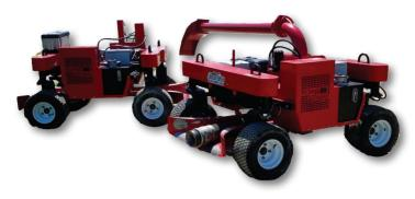
Placer Max Weight 490 lbs. per wheel Dragger Max Weight 296 lbs. per wheel
